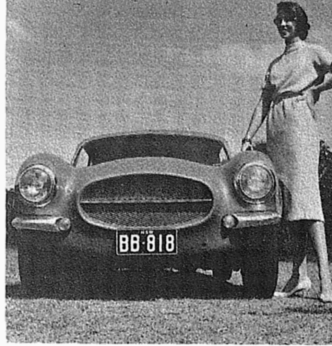
The production Buckle coupe, a shatteringly-fast GT car built around Zephyr components and selling for almost $4000. Several were raced successfully, and one is still campaigned on circuits.
