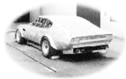
Robin Hamilton's Le Mans car in the wind tunnel at MIRA. Lessons learnt here led to Vantage bodywork.
